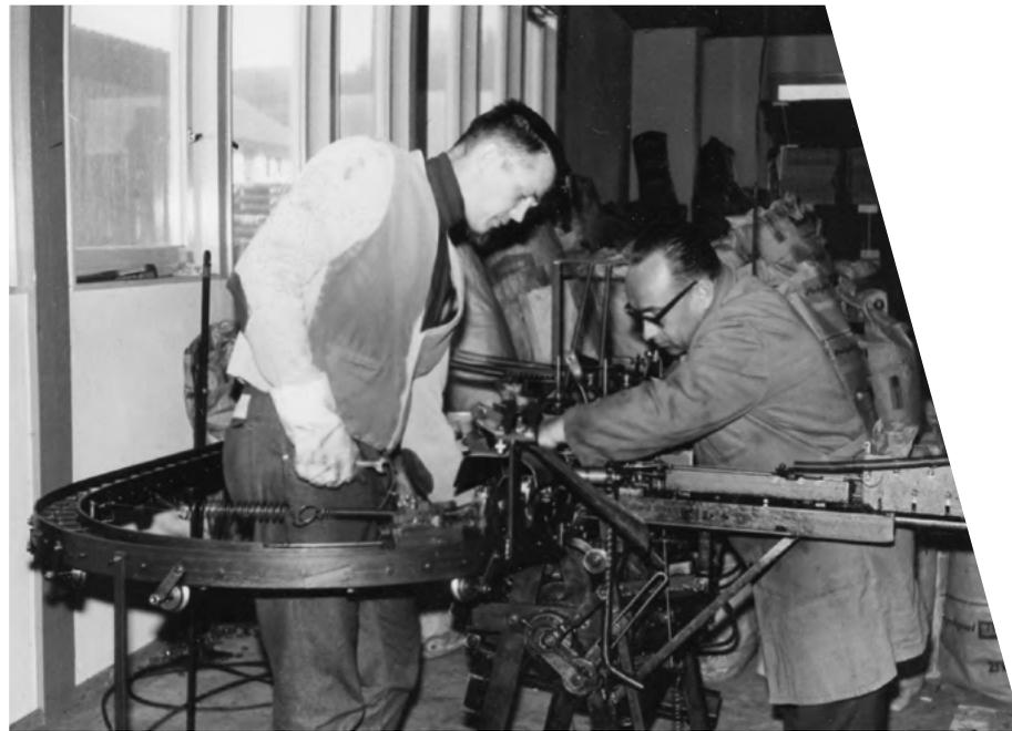
World's first machine for the production of double offset springs
